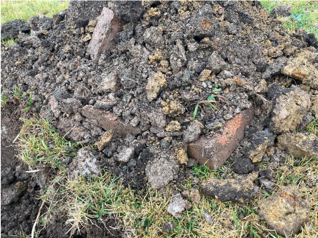
Image showing example of fill materials containing elevated concentrations of foreign materials (brick).
